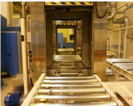
Washing machine is a part of a large conveyor system. Machine must have two pneumatic doors.
