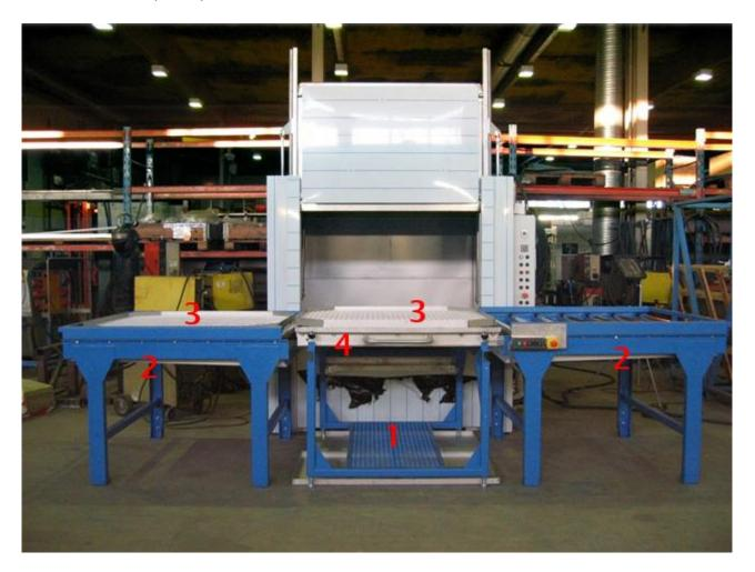
With T-roller or automatic conveyor systems, the machine becomes part of the production line, using less labor for consistent cleaning.
