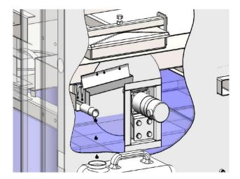
Oil will collect from the fluid surface on the rotating disc of the oil skimmer.
