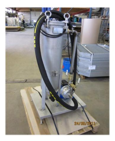
Removes of fines and oils. A pump circulates the liquid through an external filter vessel. The filter vessel is equipped with a special bag that has, in addition to mechanical filtration, the property to remove oils from the liquid flow. Depending on type of oil, up to 20-30 kg of oil can be removed with a bag. A gauge will show the pressure increase in the filter bag. The operation of the bypass filter can be continuous or connected to the cleaning cycle.
