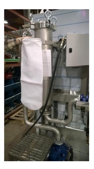
The liquid from tank is passing a fine filter unit to be. After the filter the liquid flows to the spray pipes and nozzles. The fine filter ensures that no large impurity particles can reach the pallet with its components during final rinse. Normal filter bag's filtration grade is  $25 - 50 \mu m$ .
