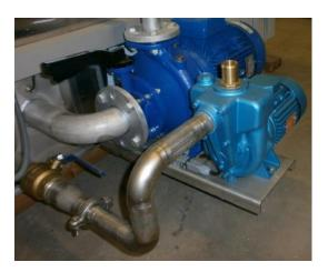
The return pump will pump the liquid back to customer's container for disposal. The pump is operated manually during service.
